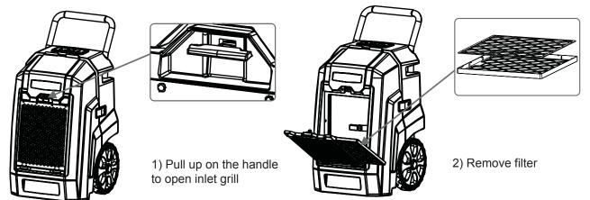
2. You can clean the filter by vacuuming it or rinsing it with warm water (no soap or solvents). Always make sure the filter is dry prior to restarting the unit.
